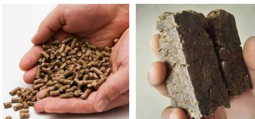
(b) *Torrefied agro-residues* – Torrefaction is a process that involves the heating of biomass in the absence of oxygen at high temperatures (typically 200 to 400°C). During torrefaction, combustible gas is released, which can be utilised for process heat. The resulting torrefied
