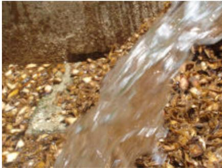
digester feedstock. As each biogas plant is completed, waste from the surrounding banana plantations is being chopped, mixed with measured amounts of water in the appropriate solid:water ratio, and inserted in the input tank, towards biogas generation.
