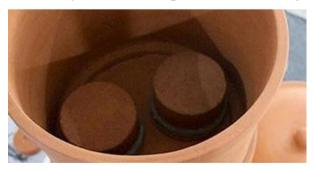
developing a water-purifier made of clay and rice-husk, with a silver-coated nano-particle disc or coin (that has to be replaced periodically). This "Swach neer Ag-Mittifil" (clean water silver-clay-filter) is designed to treat biologically-contaminated water, removing almost all impurities.
